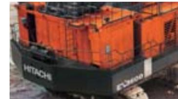
A walkway around the entire counterweight provides easy access to key rear areas. This means faster and safer inspection and maintenance.
