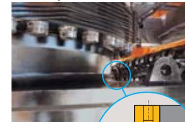
The center track frame of integral cast steel structure can avoid stress concentration and increase reliability.
