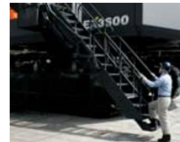
Folding stairs are designed for easy access to the machine for servicing and maintenance.
