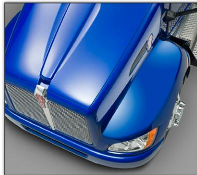
*The four-piece hood and fenders are molded from SMC, a high-tech light weight composite material for added durability and repairability.*
