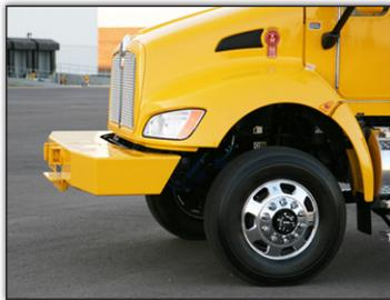
Factory installed front drive axles with capacities from 10,000 to 16,000 lbs. Non-driving front axles from 8,000 to 16,000 lbs.
