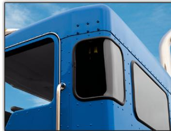
In addition to the standard peeper window in the passenger door, optional cab corner windows are available to help improve visibility in tight places.
