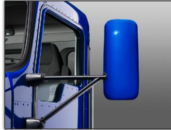
Heated and electronically-adjusted aerodynamic mirrors.
