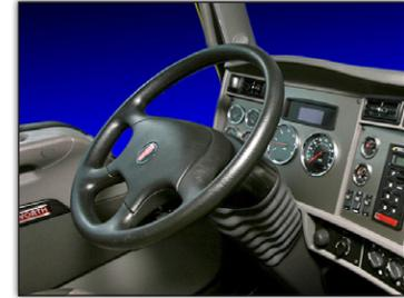
Tilt and telescoping steering column.
