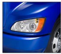
An advanced forward lighting system provides up to 30% more down-road coverage than conventional sealed beam designs. Choose the standard halogen or optional HID Xenon lamps.
