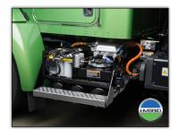
High energy lithium ion battery and controls for fuel saving Eaton hybrid system.
