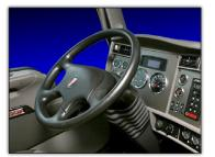
Tilt and telescoping steering column.
