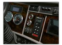
*Easy-to-operate dash control panel for Eaton automated and Allison automatic transmissions.*
