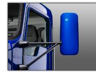
Heated and electronically-adjusted aerodynamic mirrors.
