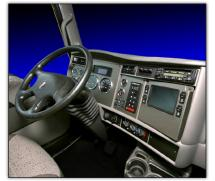
All new instrumentation with increased gauge and switch options, plus the updated gray dash panels complement the standard Pinnacle Kenworth interior. Shown with optional hybrid display.
