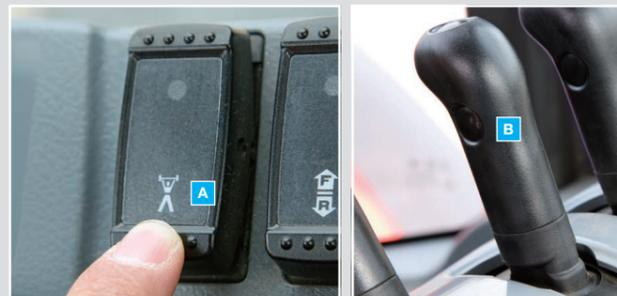
Standard mode is preselected and enough for ordinary work that requires constant power, such as loading. Power mode is selectable when extra power is needed.
