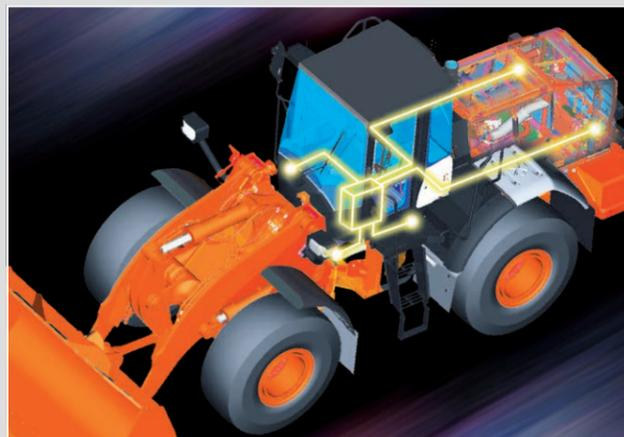
The “Active Engine Control System” plays a key role achieving a 10% fuel saving. Strategically positioned sensors detect movements throughout the machine and adjust engine speed accordingly to eliminate energy losses to maximize fuel conservation. This delivers smooth, fuel-efficient operation.
