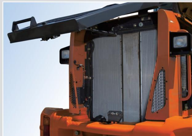
The automatic reversible cooling fan is available to keep the radiator clean at all times. The cooling fan is automatically self-reversed every 30 minutes to blow dust off the radiator. The cover swings up for efficient air blowing.
