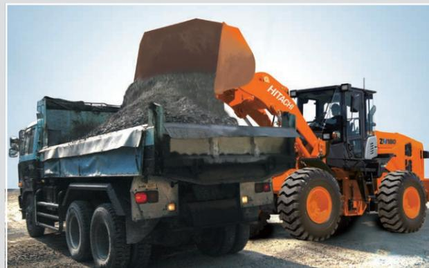
Clutch cut-off timing is adjusted by sensing travel speed and pedal depression for smooth, efficient truck loading. The Flat mode, Slope mode and OFF are selectable by switch control according to job requirements.
