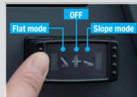
Clutch cut position switch
