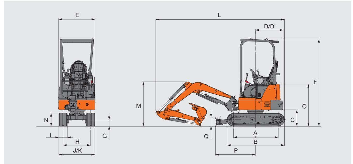
This illustration shows with 0.93 m arm, 0.044 m<sup>3</sup> bucket and 230 mm rubber shoes and heavier counterweight 240 kg.
