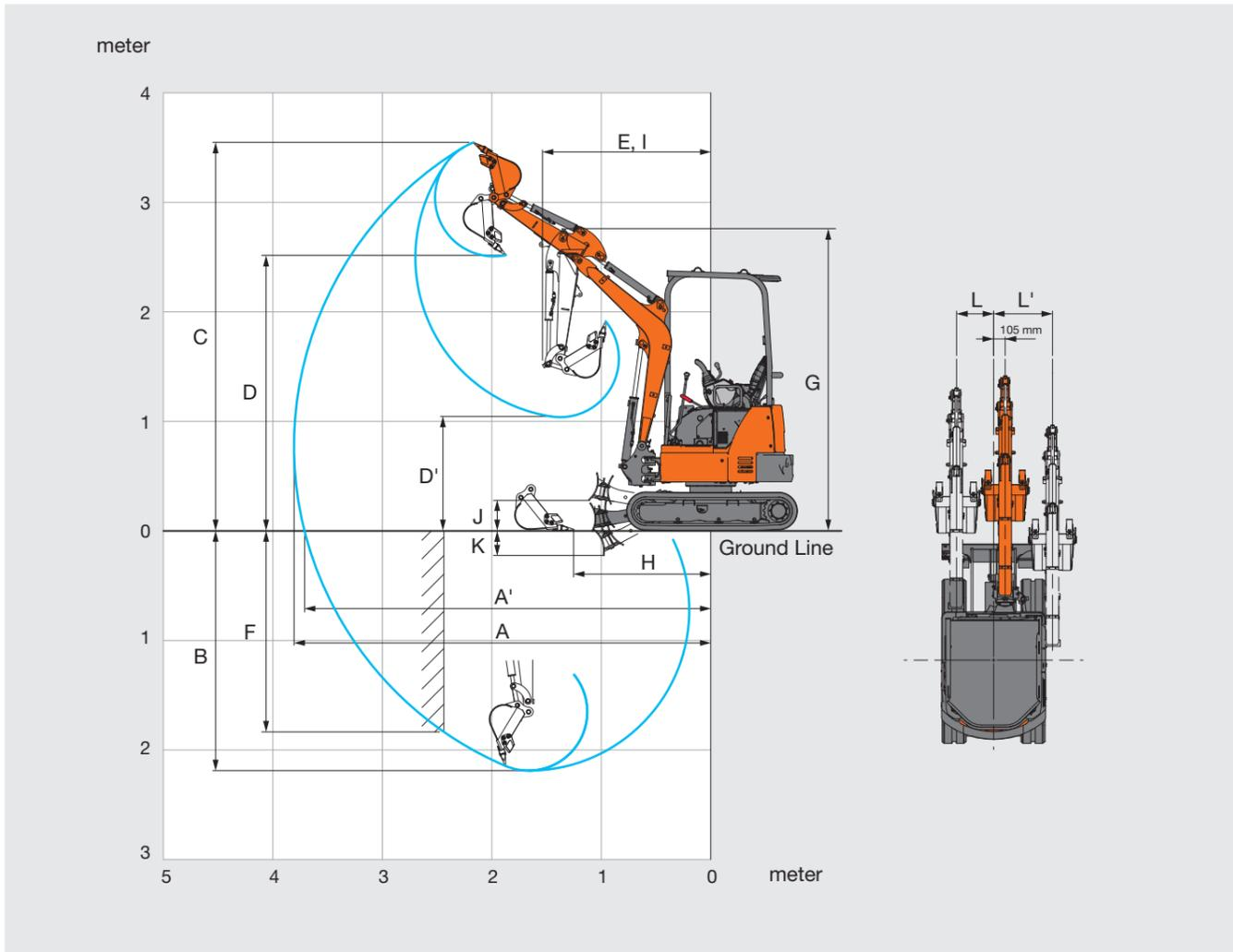
This illustration shows with 0.93 m arm, 0.044 m<sup>3</sup> bucket and 230 mm rubber shoes and heavier counterweight 240 kg.
