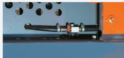
Fuel tank water drainage cock
