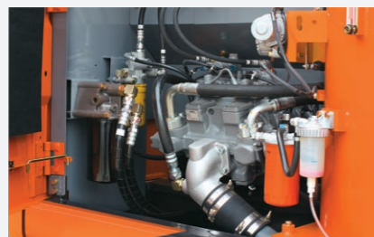
Grouped remote filters and inspection points
