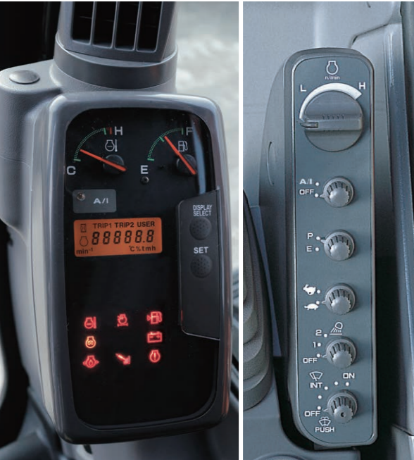
Monitor panel Switch panel
