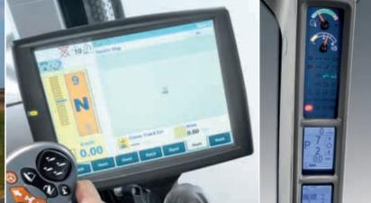
**INTELLIVIEW - GEAR AND SPEED AT A GLANCE** The standard IntelliView<sup>™</sup> IV display is configurable to provide a dedicated information panel to the left side of the screen, giving a clear read out of the selected transmission ratio and tractor speed.
